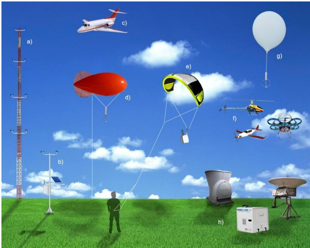
Figure 1: Platforms for wind measurement characterization. a) Meteorological mast, b) Weather station, c) MAV, d) Tethered balloon, e) Kite, f) UAVs, g) Radiosonde, h) Sodar / lidar / radar. Fonte [1].
